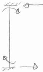
$$T_{2C} = \frac{M_{2C} + M_{21}}{c} = \frac{\frac{4EI}{c} l_2 - \frac{6EI}{c^2} \Delta_2 + \frac{2EI}{c} l_2 - \frac{6EI}{c^2} \Delta_2}{c}$$
