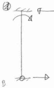
$$T_{1B} = \frac{M_{1B}}{c} = \frac{\frac{3EI}{c} l_1 - \frac{3EI}{c^2} \Delta_2}{c} = \frac{3EI}{c^2} l_1 - \frac{3EI}{c^3} \Delta_2$$
