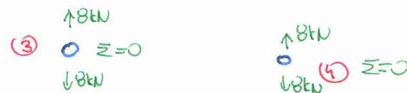
$$T_{③} = R_{③} = 4 \text{ kN}$$
